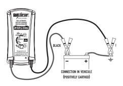
If Positively Earthed – FIRST Connect the Black (-) Crocodile clip or optional ring terminal lead to the (-) battery terminal and then connect the Red (+) Crocodile clip or optional ring terminal lead to the vehicle's chassis. DO NOT connect the Red (+) lead to the carburettor or fuel lines.
