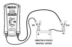
If the battery is still **in the vehicle**, determine if the vehicle is positively or negatively earthed. If **Negatively Earthed (Most Common)** – FIRST Connect the Red (+) Crocodile clip or optional ring terminal lead to the (+) battery terminal and then connect the Black (-) Crocodile clip or optional ring terminal lead to the vehicle's chassis. DO NOT connect the Black (-) lead to the carburettor or fuel lines.
