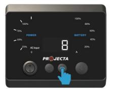
Step 3. Long press the scroll down/confirm button for 2 seconds to trigger on the configuration, the number/icon will flash.
