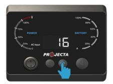
Step 5. Afterwards, long press the scroll down/confirm button for 2 seconds to confirm the configuration. The two bars (load ratio and battery soc) will flash indicating the configuration is in process.
