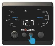
Step 1. To enter into the configuration: Press scroll down/confirm button for 2 seconds.
