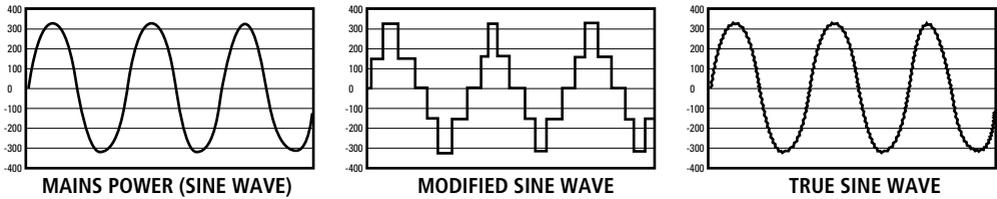
Logically it follows that the process used in a true sine wave inverter is more complex than a modified sine wave inverter and subsequently they are lot more expensive.
