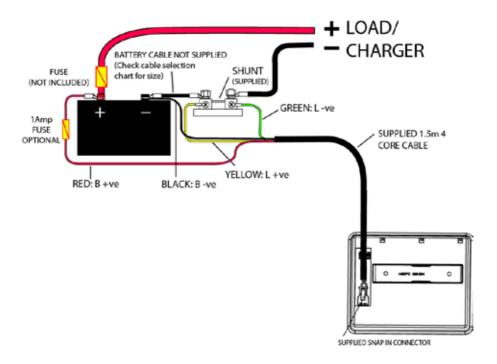
**NOTE:** There should only be one cable connected to the battery negative terminal. This should be to the battery side of the shunt to ensure all load is measured through the shunt. All other NEG/Earth connections should be made at a load side of the shunt.
