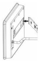
Close the battery monitor onto the clip until you hear the "click" sound. Make sure that the cable assembly has been fed into the hole correctly.
