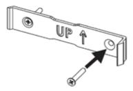
Drill a 15mm Diameter hole 20mm from the screw hole as pictured to allow the connector to pass through.
