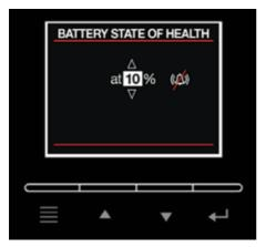
The battery state of health diminishes to the set level, an audio alarm is activated. The audio alarm can be muted by pressing any buttons.
