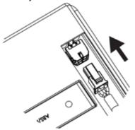
Feed the cable through the pre drilled hole and slide the left hand side of the battery monitor into the bracket tab.
