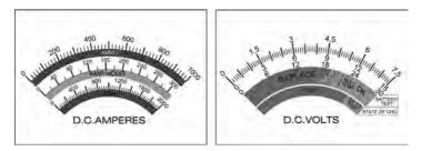
Note: Battery ouput varies due to temperature change, the 'Battery Test' scale has four temperature calibrations (21°, 10°, -1° and -18° Celcius). Use the closest scale to the approximate ambient temperature.
