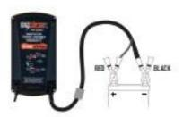
If the Battery is **out of the vehicle:**Connect the Red/Orange (+) Crocodile clip or ring terminal to the positive (+) battery terminal.
