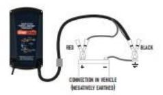
If Negatively Earthed (Most Common) – FIRST Connect the Red/Orange (+) Crocodile clip or ring terminal lead to the positive (+) battery terminal and then connect the Black (-) Crocodile clip or ring terminal lead to the vehicle's chassis or negative (-) battery terminal. DO NOT connect the Black (-) lead to the carburettor or fuel lines.
