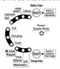
**Note:** If the Battery Type and Charge Rate LED's are both flashing, this indicates no battery is detected or is below 2V and the unit is in Eco Power Saving mode.
